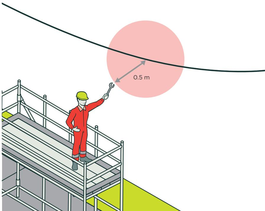
**FIGURE 4:** Worker with consent to work up to 0.5 m from the low voltage overhead electric line
